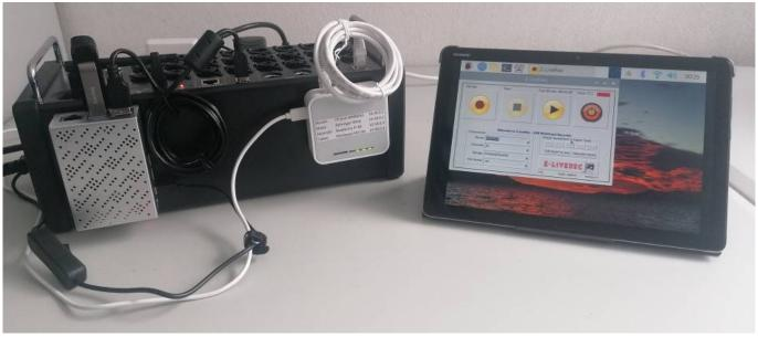
The XR18 has the RPi attached at the left side with klett stripes, an the access point to the right. I can easy switch between Z-LiveRec and Mixing Station by swiping (swipe down from top and select the other app). Both apps keep running all time.
